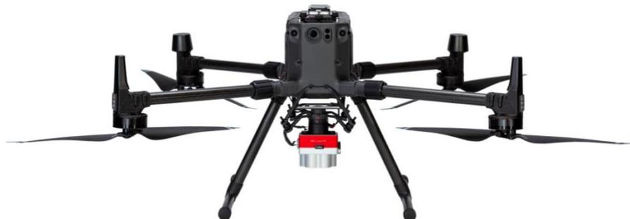
Altum-PT and DLS 2 on a Matrice 300. The sensor draws power directly from the Matrice via the Skyport.
