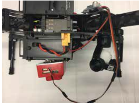
XT30connector plugged into distribution board
