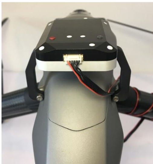
Showing DLS2 mast mounted on Inspire 2 with DLS 2 connector facing forward
