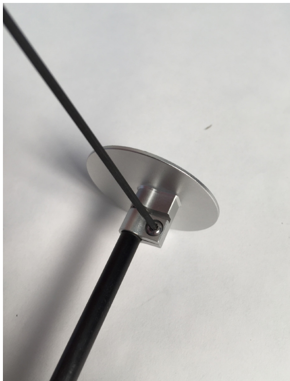
M2 screw being tightened on mast assembly
