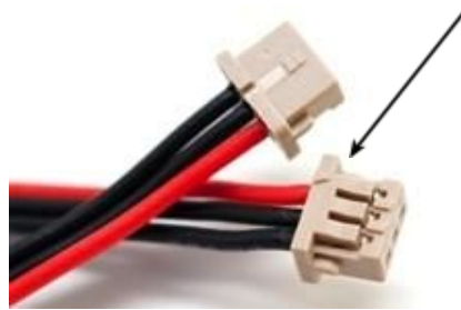
Pin 1 indicator on DF13 family of connectors (DF13-3S-1.25C shown)
