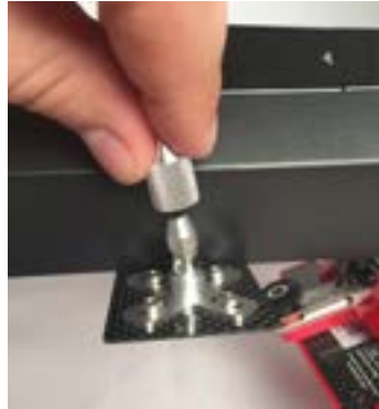
The locking mechanism on the mast will need to be tightened.
