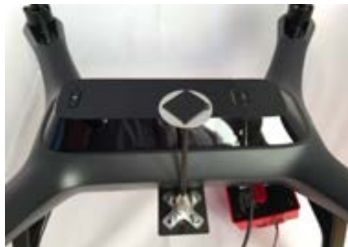
VHB tape applied to the top of the cleaned mast.
