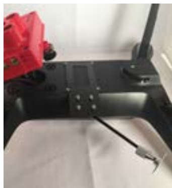
Mast and mast mount attached to the Solo.
