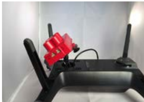
Camera tilted to compensate for tilt during flight.
