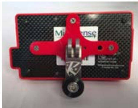
Three flat head screws tightened to the RedEdge.
