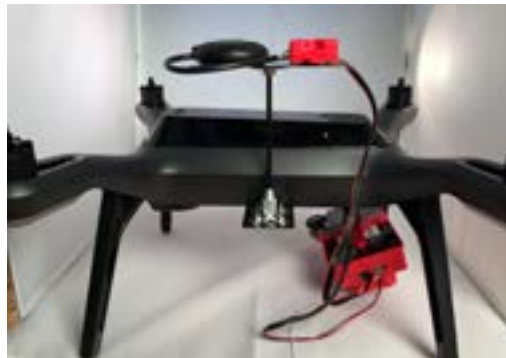
6pin cable connected between the RedEdge and DLS.
