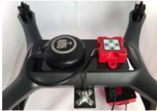
GPS and DLS mounted with VHB and connected with their associated cables.
