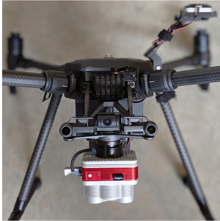
Altum and DLS 2 on a Matrice 200. The sensor draws power directly from the Matrice via the Skyport. The DLS 2 is the highest object on the aircraft.
